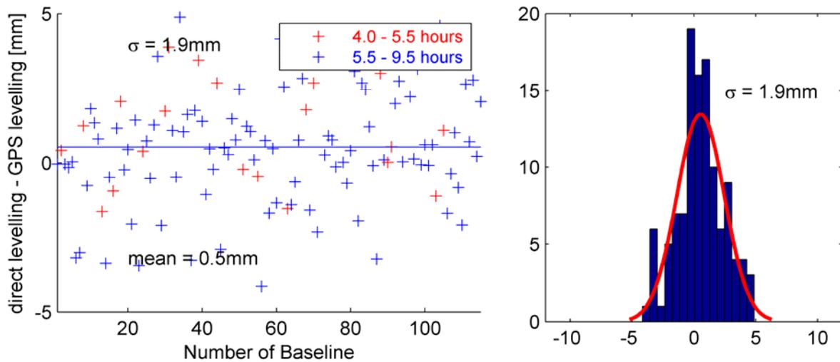
**Fig. 7: Differences between GPS and precise leveling (L2)**
