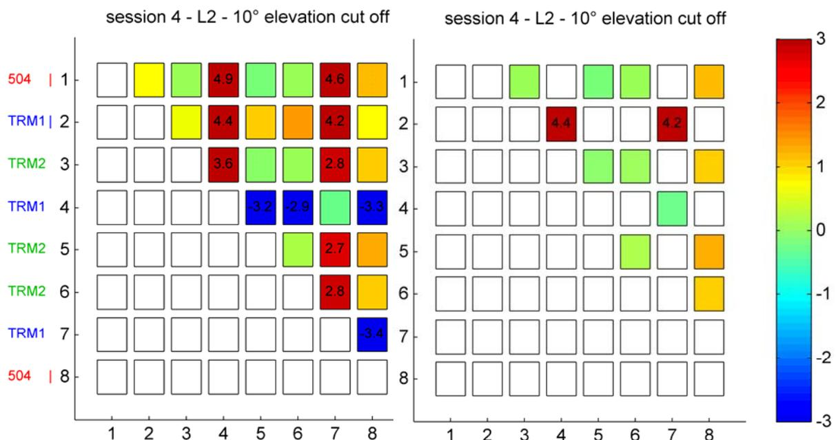
**Fig. 10: Differences between GPS and precise leveling (L2) – Session 4**
