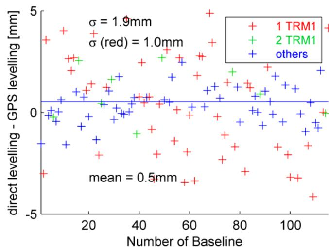
**Fig. 12: Differences between GPS and precise leveling (L2) with highlighted near-field effects**
