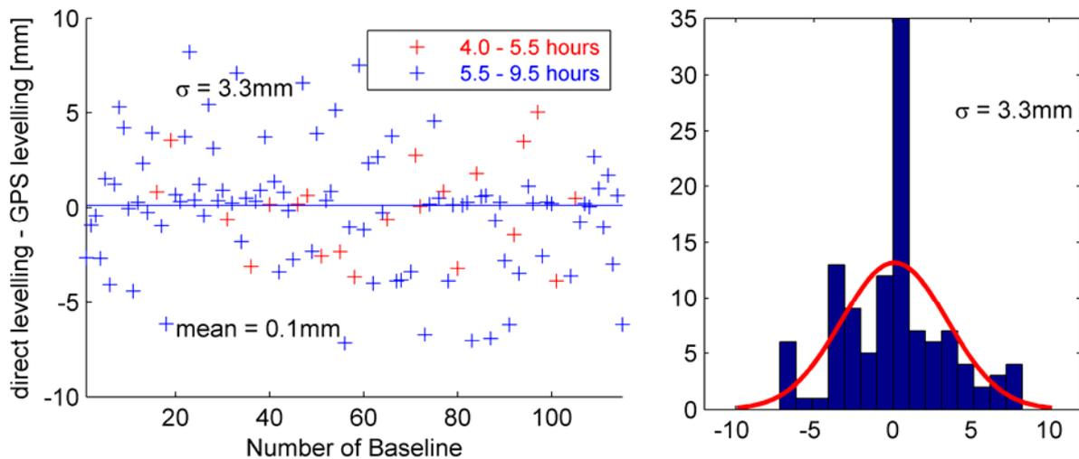
**Fig. 8: Differences between GPS and precise leveling (L0)**
