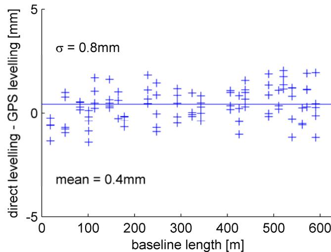
**Fig. 6: Differences between GPS and precise levelling (L1) - sorting: baseline length**
