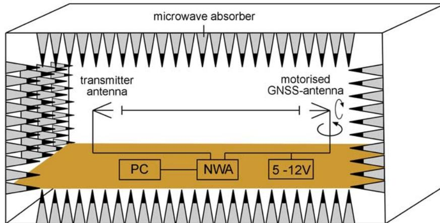
**Fig. 2: Setup of the anechoic calibration facility (Zeimetz and Kuhlmann 2008).**
