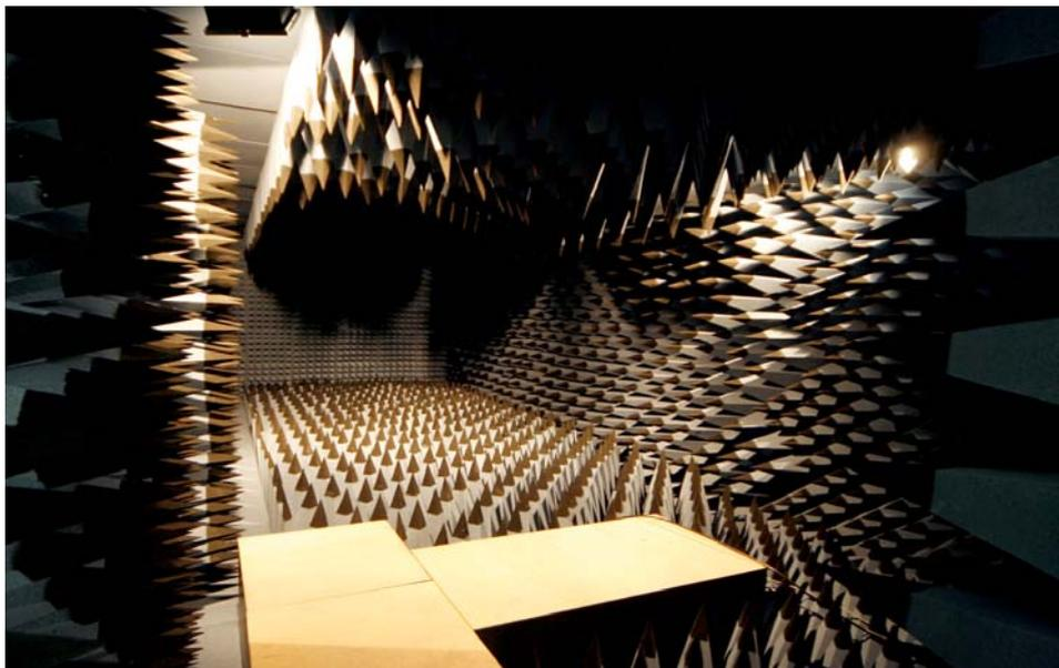
**Fig. 3: Antenna calibration laboratory Bonn (without antenna positioner)**
