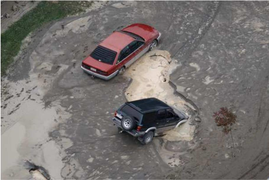
**Figure 6: Area of liquefaction in Christchurch**
