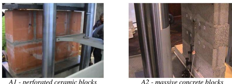
*A1 - perforated ceramic blocks* *A2 - massive concrete blocks*
