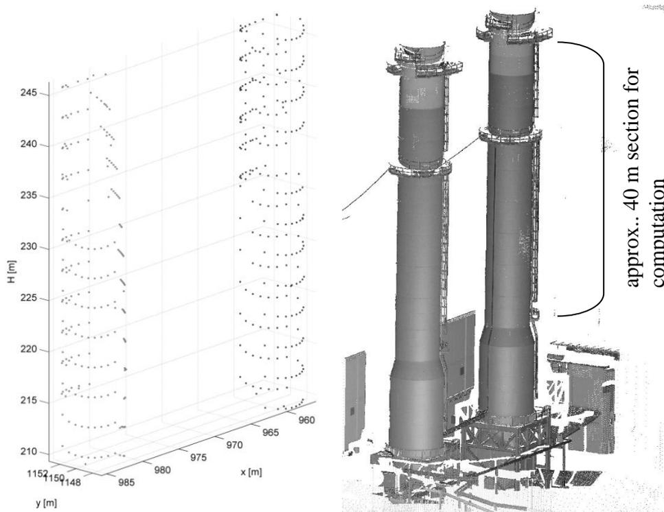
Fig. 3 Point clouds achieved by Leica Geosystems TS30 R1000 (left) and Riegl VZ-400 (right, with marked section for computation).
