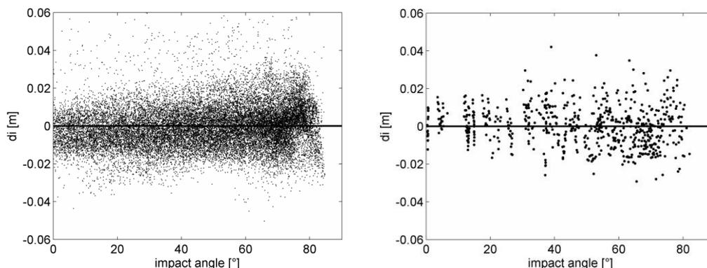
Fig 6 Dispersion of points on the chimneys surface (left – TLS, right – TPS).
