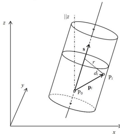
Fig. 1 Inclination of the chimney's axis – cylinder parameters.
