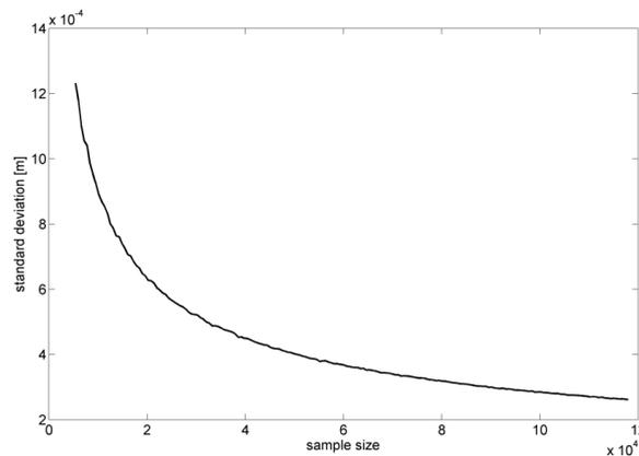
Fig. 5 Dependency of the inclination precision according to the sample size.
