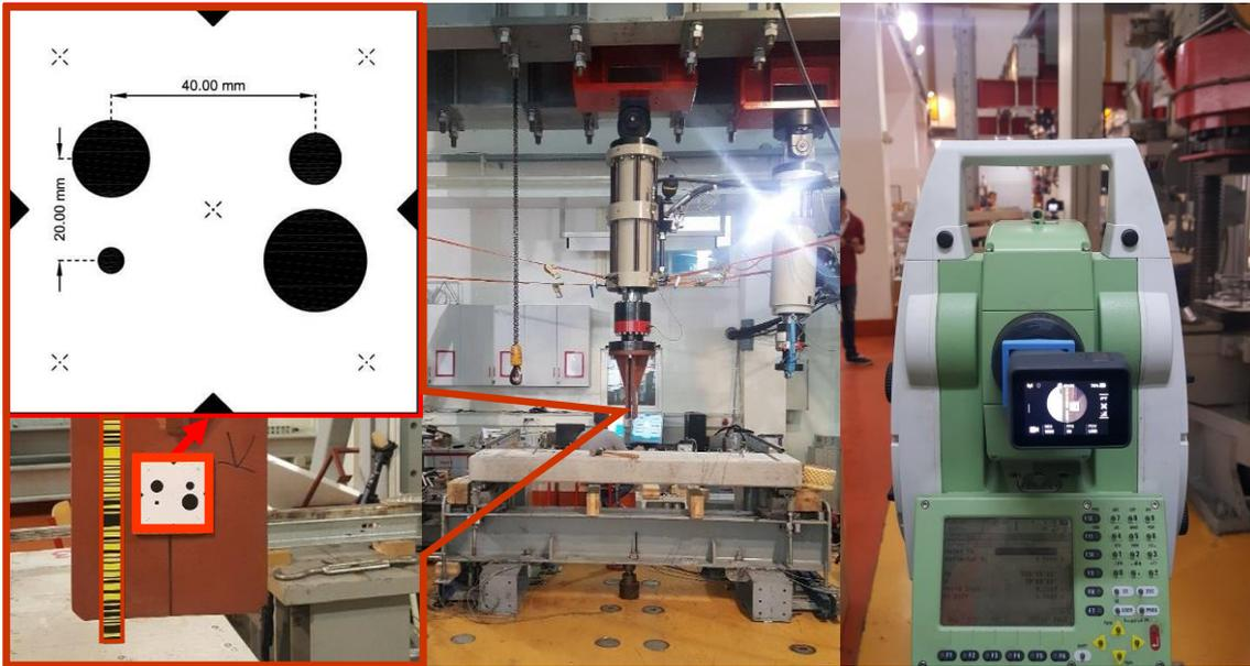
*Fig. 2 Signal marks-barcode and photomark (red on the left), testing machine (middle) and IATS prototype (right)*
