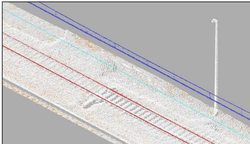
Fig. 8 Classified point cloud. Rails (red), catenary (blue), ground (orange), noise (turquoise)
