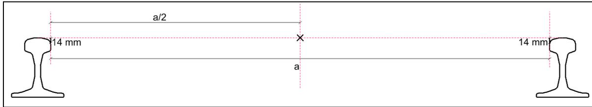
Fig. 1 Determination of rail track centre.  $a$  – nominal rail spacing
