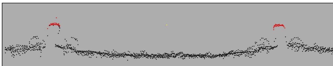
Fig. 12 Correctly determined rail track centre with single point noise on the left
