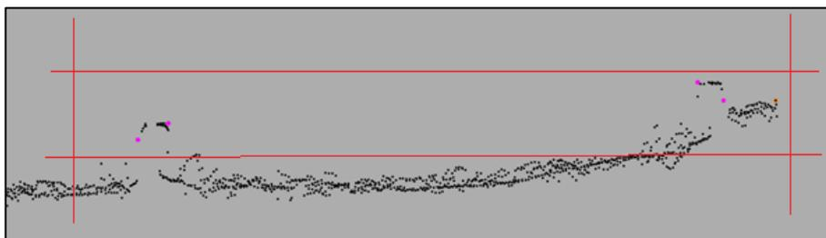
Fig. 4 Limiting search for rail heads vertically and horizontally within point cloud section
