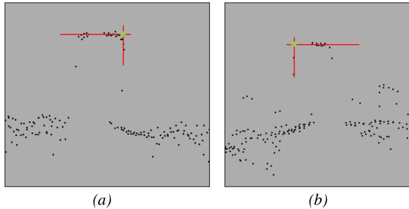
Fig. 9 Lines fitted to top surface and inner surface of railhead (left (a) and right (b)).
