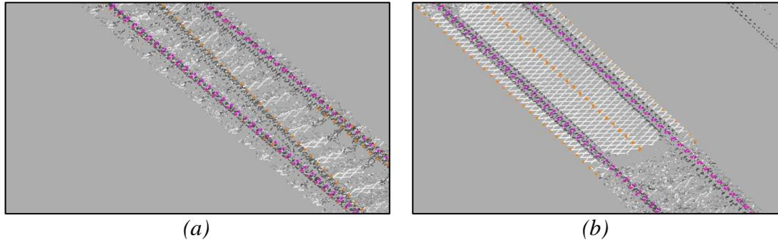
Fig. 7 Corrected bounding boxes (pink) against first determined bounding boxes (orange) on a turnout (a) and a crossing (b)
