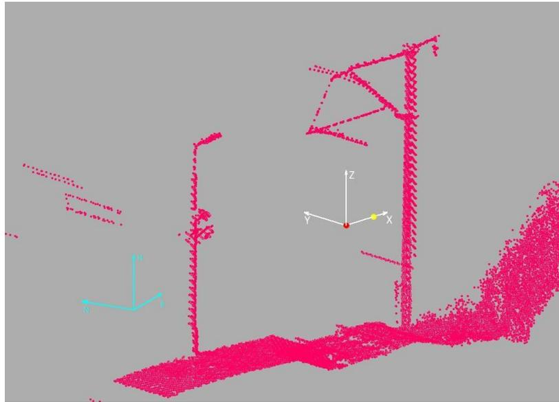
Fig. 3 Sample point cloud section, global coordinate system (teal), section local coordinate system (white), section key point (red), section directional point (yellow) (Pastucha, E. 2016)
