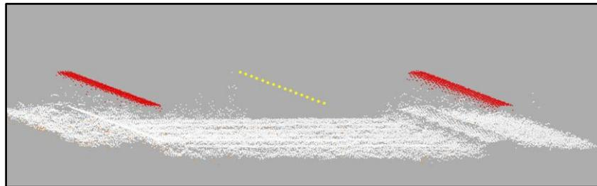
Fig. 10 Determined rail track centre (yellow) against classified point cloud (rails – red)
