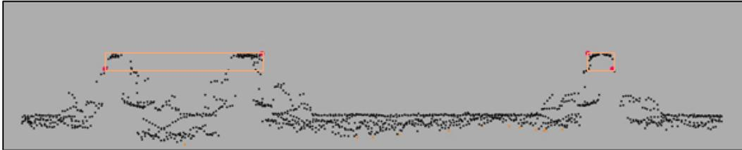
Fig. 5 Calculated bounding boxes against their point cloud section
