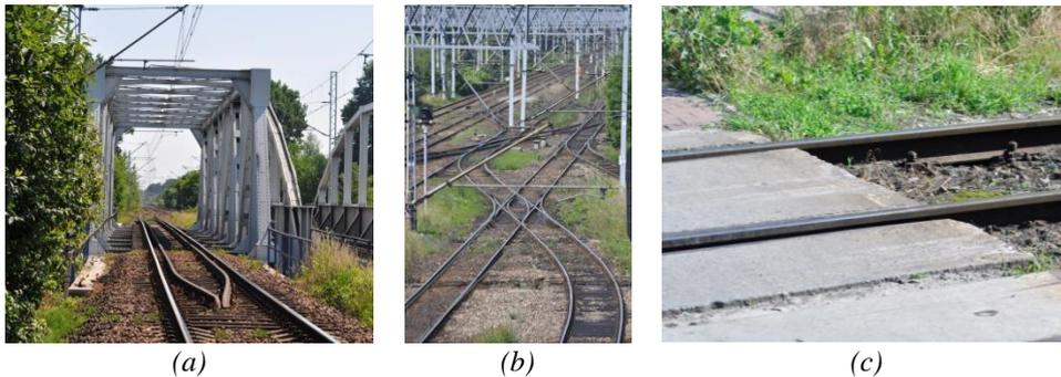
Fig. 6 Check rails (a), turnouts (b) and railway crossings (c)
