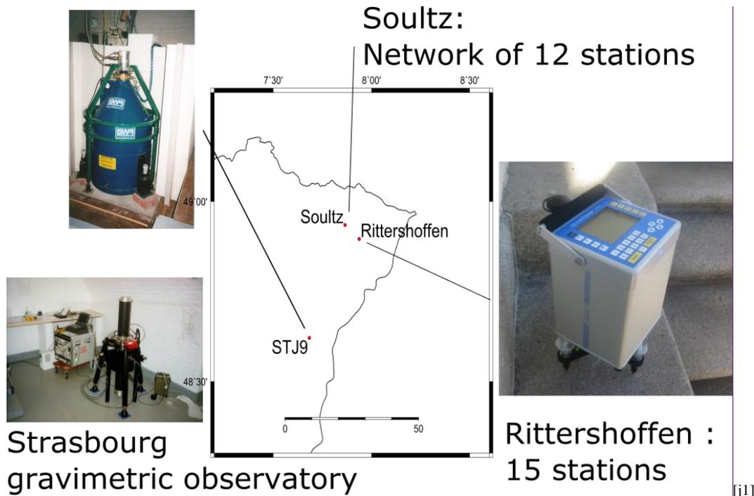
*Fig. 2 The three main locations of our hybrid gravity approach. STJ9 is the Strasbourg Gravimetry Observatory where both a superconducting gravimeter (GWR C026) and an absolute gravimeter (Micro-g Solutions FG5#206) are available. There are 12 micro-gravity stations in the Soultz network (GEIE) and 15 stations close to Rittershoffen (ECOGI) (modified from Hinderer et al 2015).*
