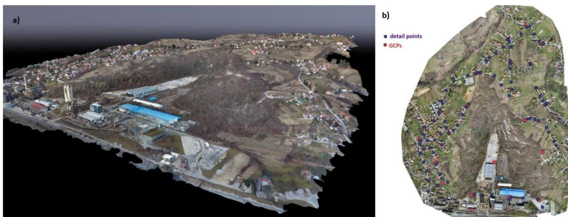
Fig. 4 Point cloud (a) and ortho-mosaic with position of GCPs and detail points (b) of the landslide
