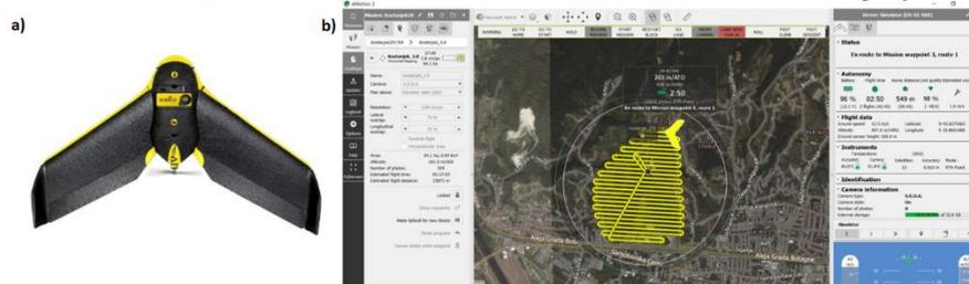
Fig. 3 senseFly eBee RTK (a), the flight plan in senseFly eMotion3 software (b)
