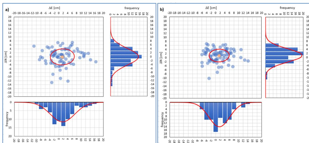
Fig. 6 Distribution of displacement errors (epoch III – epoch I) for Method 1(a) and Method 2 (b)
