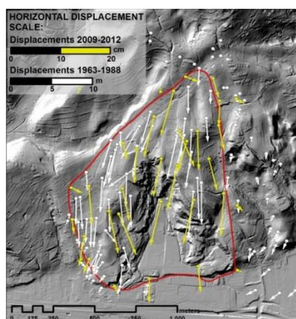
*Fig. 1 Comparison of horizontal displacements determined between 2009. - 2012. (yellow arrows) and 1963. - 1988. (white arrows) (Mihalić Arbanas, S. et al. 2016)*
