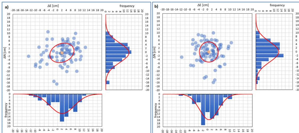
Fig. 5 Distribution of displacement errors (epoch II – epoch I) for Method 1(a) and Method 2 (b)
