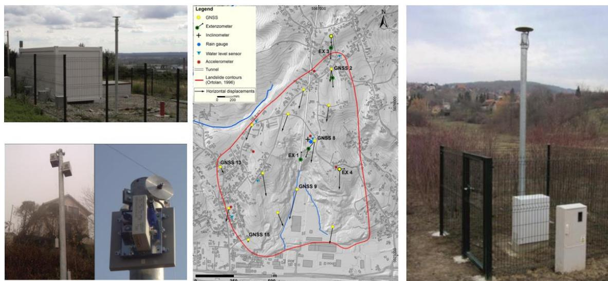
Fig. 2 Monitoring sensors at the Kostanjek landslide, their location, and the horizontal displacements recorded by the GNSS sensor network from January 2013 to January 2015 (Krkač, M. 2015).
