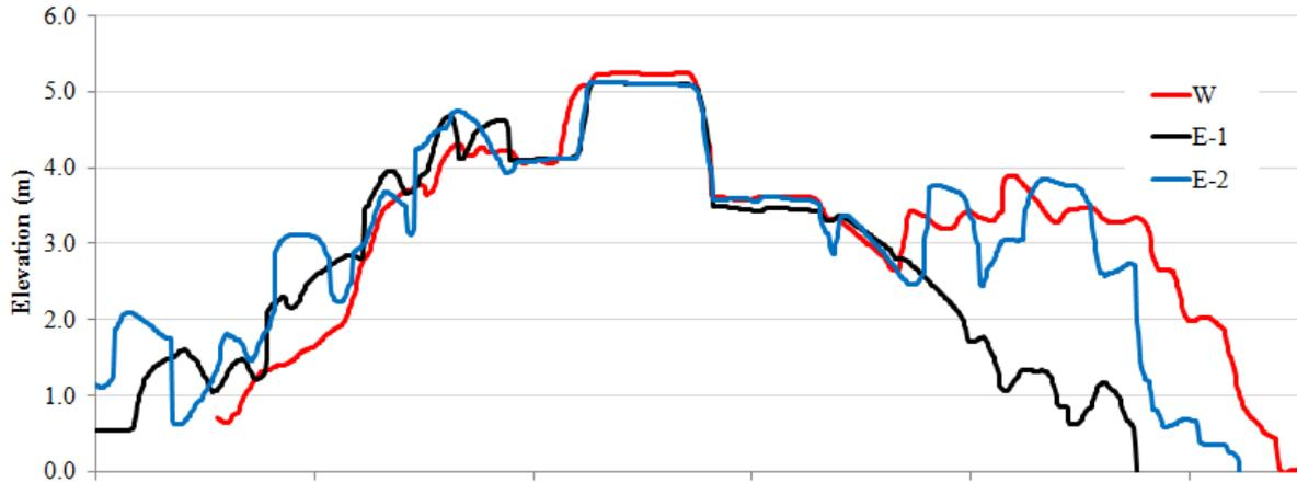
Fig. 13 Portimão breakwaters: one profile of the west (W) breakwater and two profiles of east (E) breakwaters
