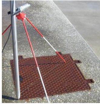
*Fig. 9 Corner of a manhole being coordinated*
