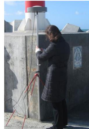
*Fig.10 Coordinating a point by GNSS*
