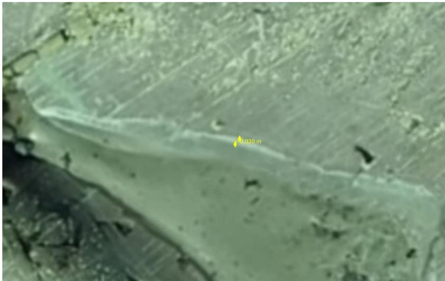
*Fig. 6 A maximum thickness of the same joint as in fig.5 could be determined at a level of detail better than 3 cm (Tziavou, 2016)*
