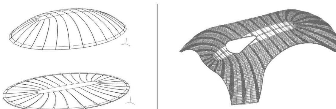
Fig. 1 Schematic sketch before (left, below) and after (left, above) lifting process; CAD plan of the pavilion (right)
