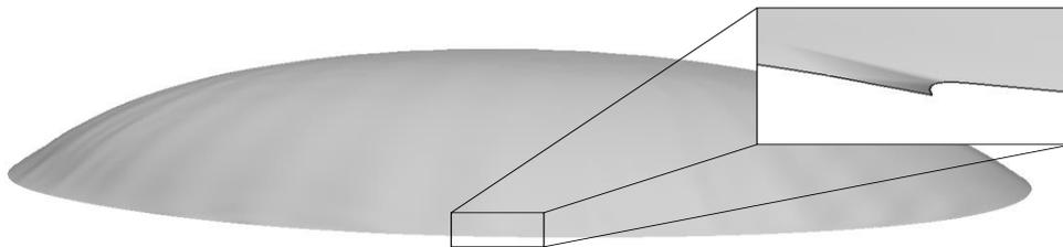
*Fig. 5 Approximation of the B-Spline surface with artefact on the bottom edge*
