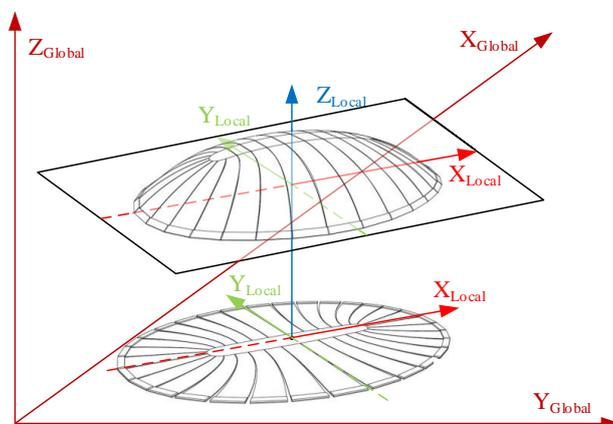
Fig. 3 Schematic sketch of the local and global coordinate system definition
