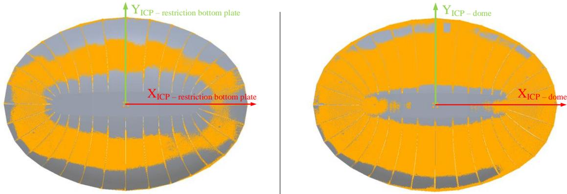
Figure 4: ICP datum differences. ICP – ground plate restriction (left, see 4.1.1); ICP - dome (right, 4.1.2); grey: CAD model; brown: the scanned 3D point cloud
