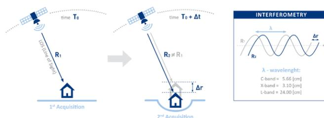
*Fig. 1 Schematic showing the relationship between ground displacement and signal phase shift*
