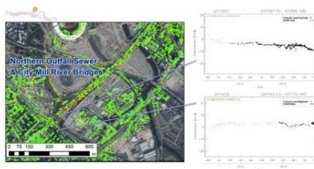
Fig. 8: Selected time series from the correlation study of both techniques on Northern Outfall Sewer & City Mill River Bridges.
