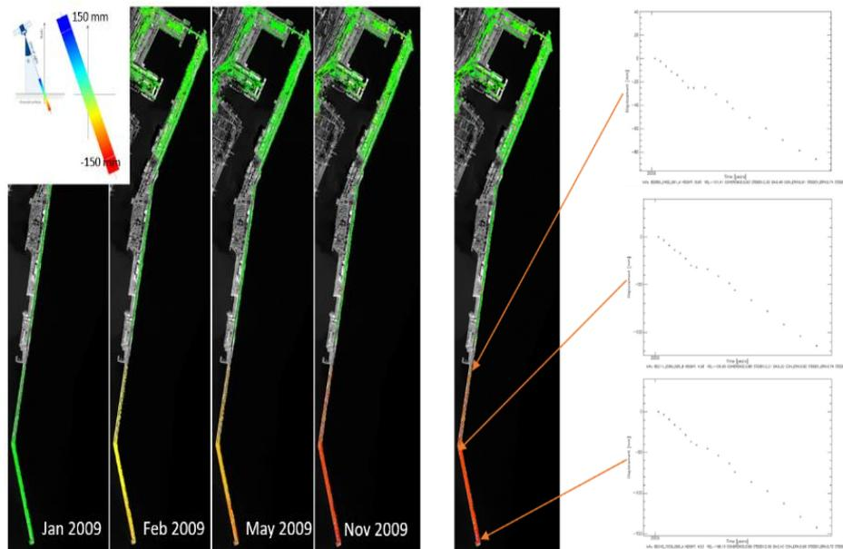
Fig. 5 Left Temporal evolution of the settlement in LOS (Line of Sight of the satellite) in the eastern dike with TerraSAR-X. Right: TS over the eastern dike with TerraSAR-X.
