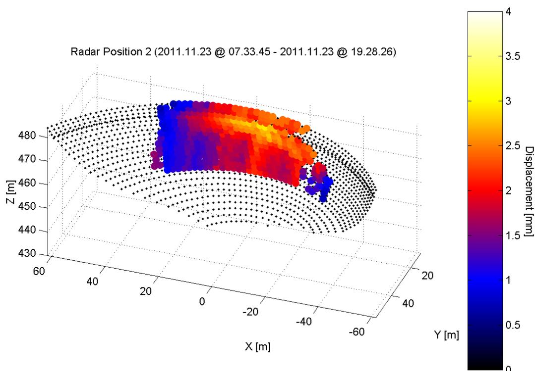
Fig. 2 Map of dam displacements rendered on the dam surface
