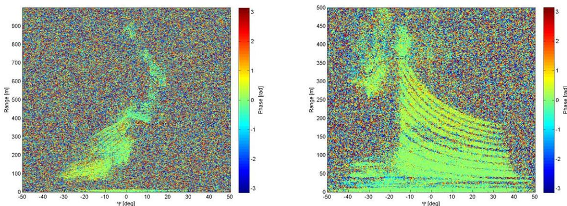
Fig. 5 Ground-based interferometric SAR data of the area around the Occhito dam. From the top to the bottom: SAR amplitude, interferometric coherence and interferometric phase. Data are referred to the left (left column) and right (right column) views of upstream surface and have been acquired on 03/03/2014
