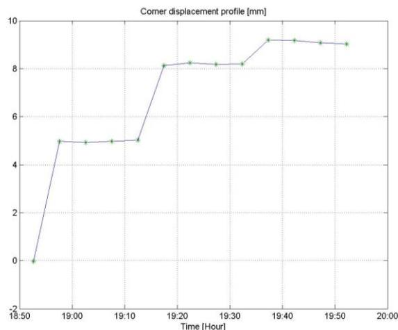
*Fig. 1 Displacements of corner reflector measured by GBSAR interferometry vs acquisition times of SAR images*
