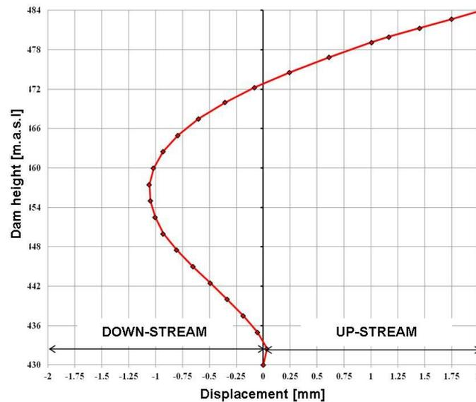
Fig. 4 Dam displacement at the centerline simulated by the SAP 2000. Displacement are referred to the time interval between the first and the second campaign.
