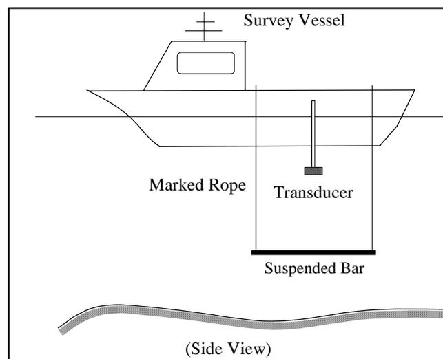
**Figure 1.** Schematic Depiction of Bar Check Calibration
