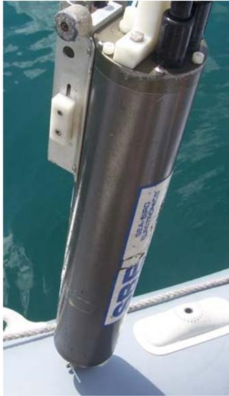
**Figure 3.** CTD Instrument (*from second application*)
