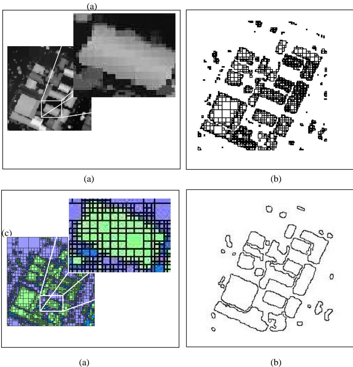
**Figure 5** – Result of the DEM segmentation using the proposed methodology. (a) Result of recursive splitting. (b) Contour obtained by the recursive splitting. (c) Region merging result (d) Contour obtained by region merging.
