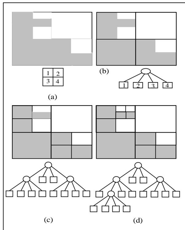
**Figure 2** – The building of a quad tree. (a) Original Image. (b) Original splitting into four subregions (the left node in the tree corresponds to the top left region in the image). (c) Splitting the regions from (b) into four subregions. One of these regions is still a gray region. (d) Splitting of the last gray region and the final quad tree (Source: Adapted from Jain et al., 1995).
