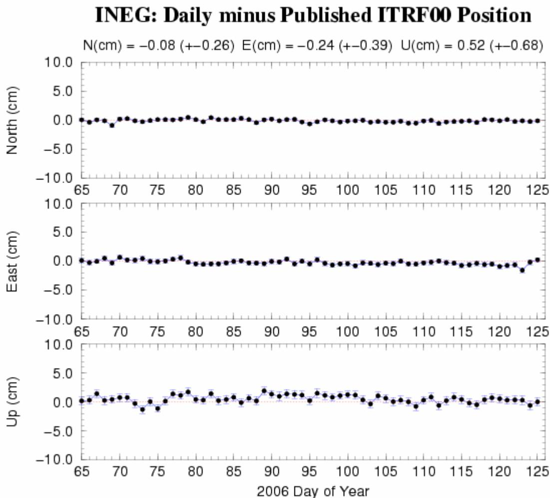
**Fig. 3** Variation of coordinates at the INEGI site during a time period of 60 days
