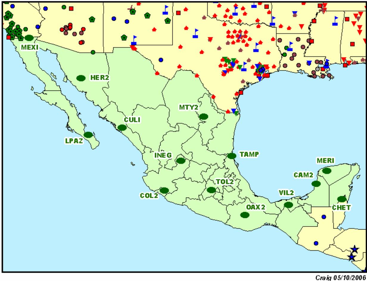
**Fig. 1** Active control stations and/or CORS in and around Mexico.
