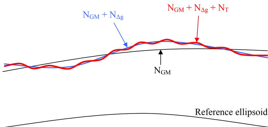
Figure 1. Gravimetric geoid undulation.
