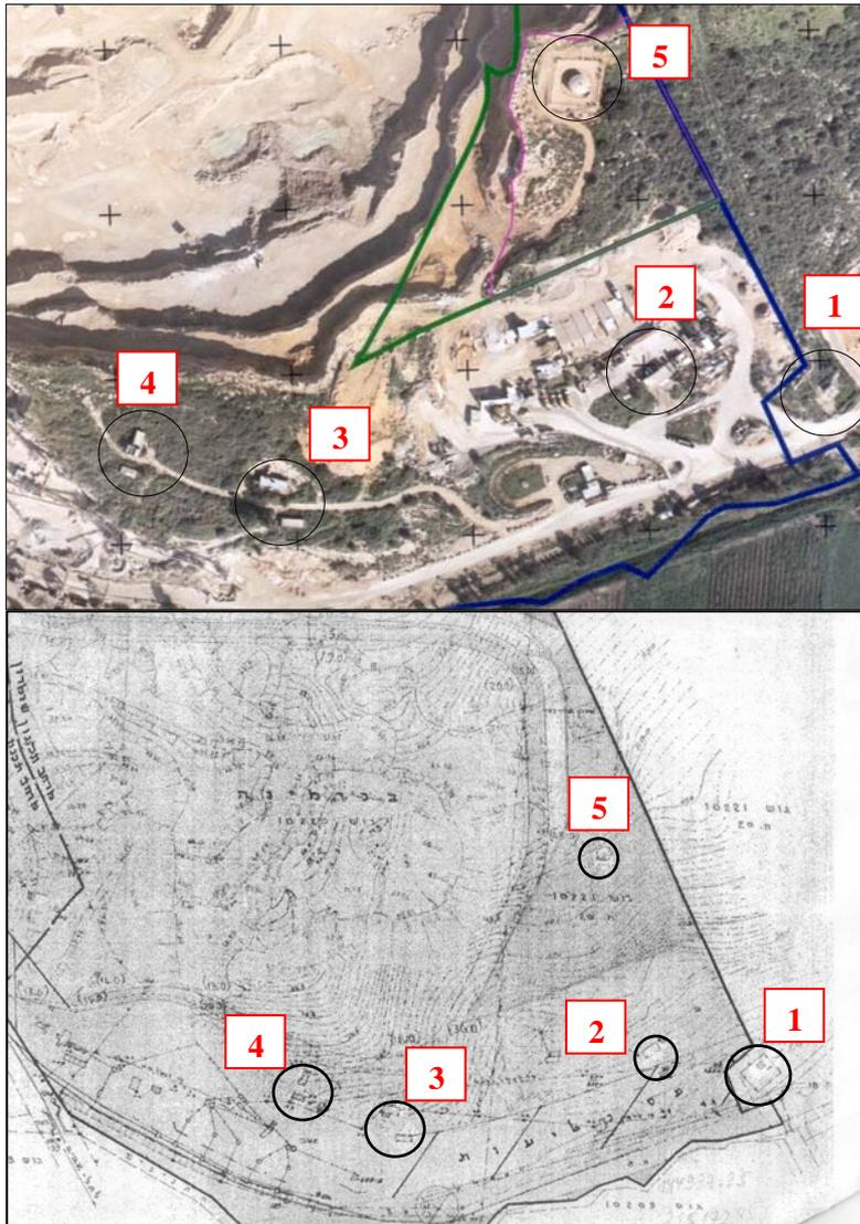
**Figure 2:** Case 2, the Shoni quarry in Binamina. At the top, the different topographic features used to position the map, bottom the Urban Construction Plan and the various topographic features identified.
