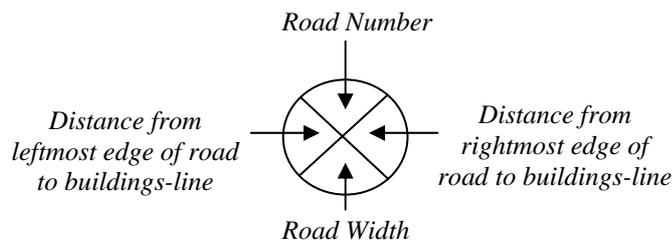
**Figure 3** : A special symbol used in Urban Construction Plans to define the ROW.
