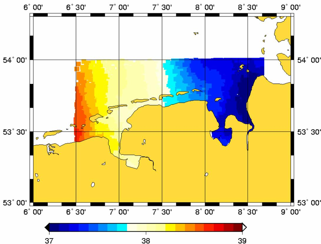
**Fig. 7** Chart datum heights above the ETRF89 ellipsoid on the East Frisian coast.
