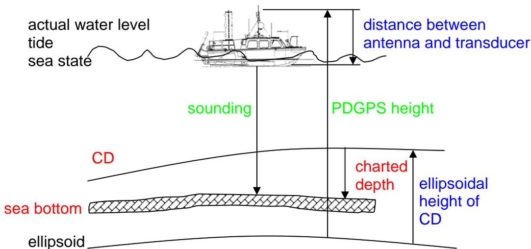
**Fig. 4:** Quantities to be considered when GNSS is used for tide correction
