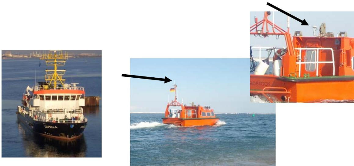
**Fig. 10:** Survey vessel CAPELLA and the antenna position on her launch.
