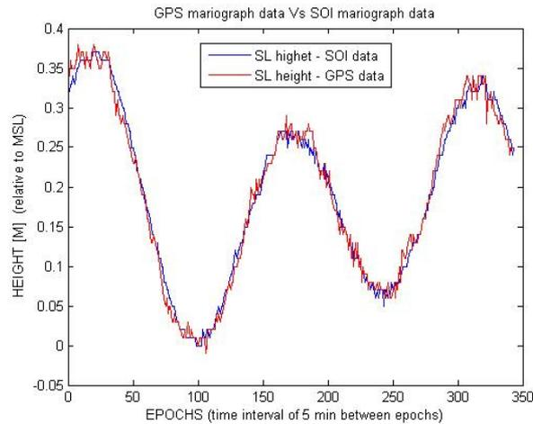
**Figure 4** – Comparison of SOI-TG data versus the GPS mariograph data.
