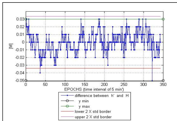
**Figure 5** – Difference between normalized GPS measurements and SOI.
