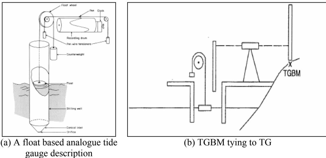
**Figure 1-** The operation principles of float based tide gauge (figures adapted from IOC 85).
