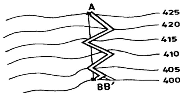
**Fig. 7** – The mapping out of a winding road in a vineyard
