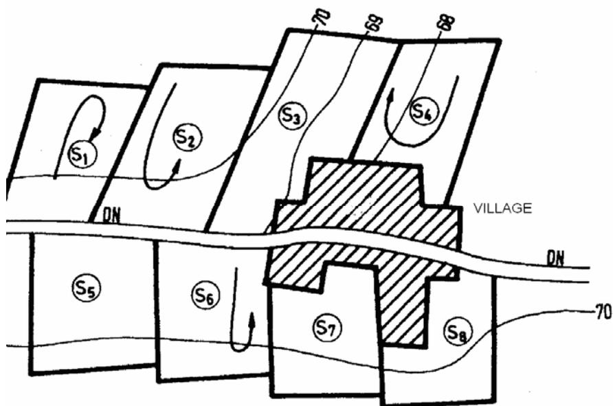
Fig. 4 – Linear placement of plots
