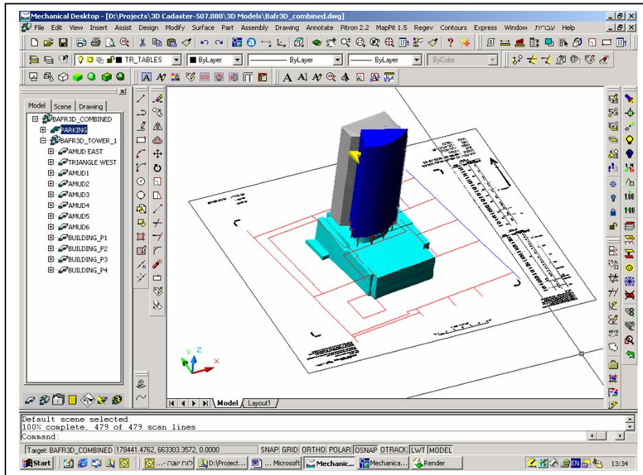
**Figure 1:** A multistory building – The land parcels regarding to the parking and a 3D model of the building and the parking (*By courtesy of Mr. Ronen Grinstein*).
