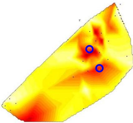
**Figure 6:** The variations of deformations of the local control network of Tranås, based on the residuals shown in figure 5. The deformations are weighted inversely to the square of the point distance. The two marked common control points were deviant, and finally excluded.
