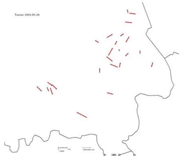
**Figure 5:** The residuals after transformation of control points with RIX 95 transformation parameters.
