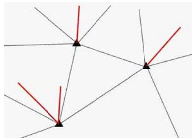
**Figure 4b:** The residual from one control point is then moved along the triangle side to do a vector subtraction.
