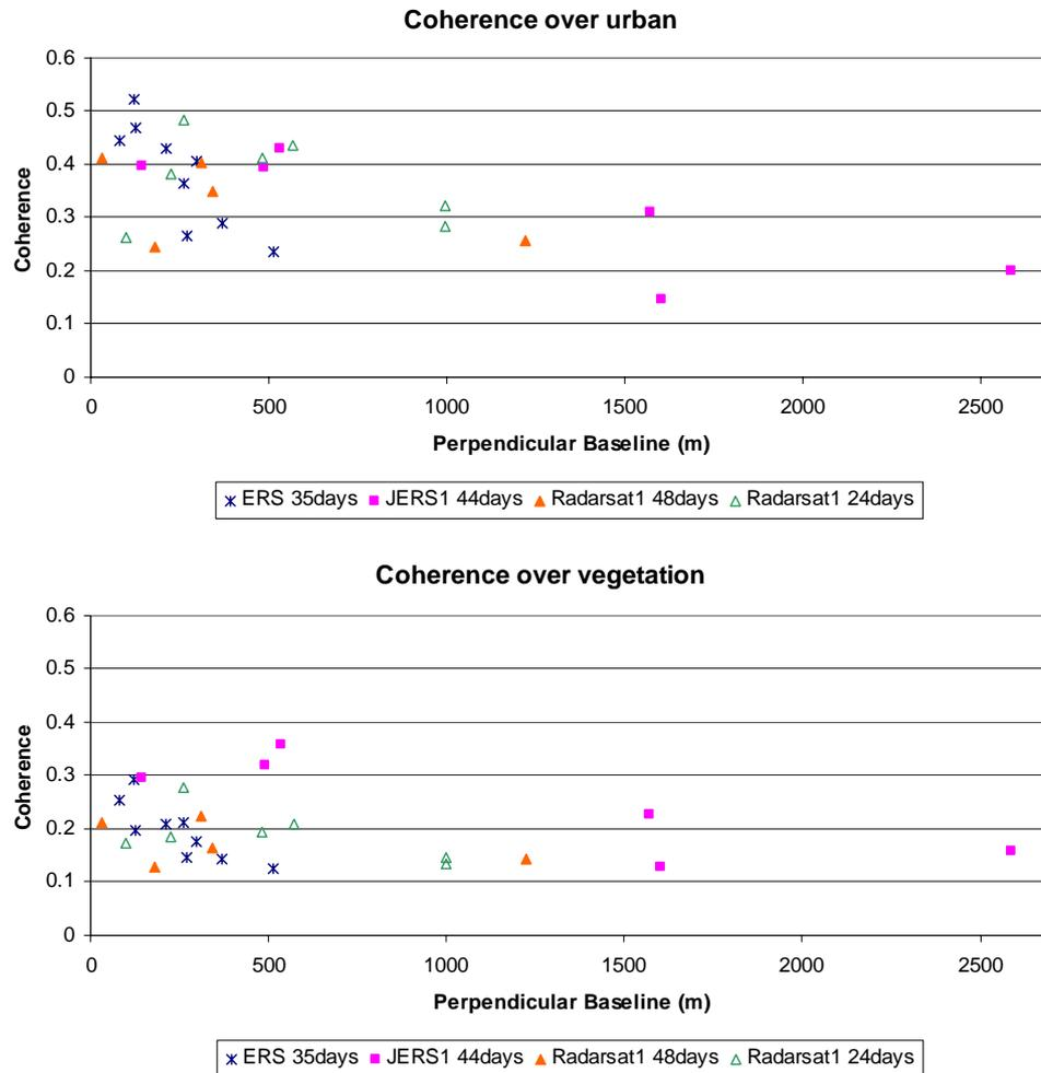
**Figure 3.** The coherence of the interferometric pairs of ERS-1/2, JERS-1 and Radarsat-1 for (top) urban and (bottom) vegetation regions.
