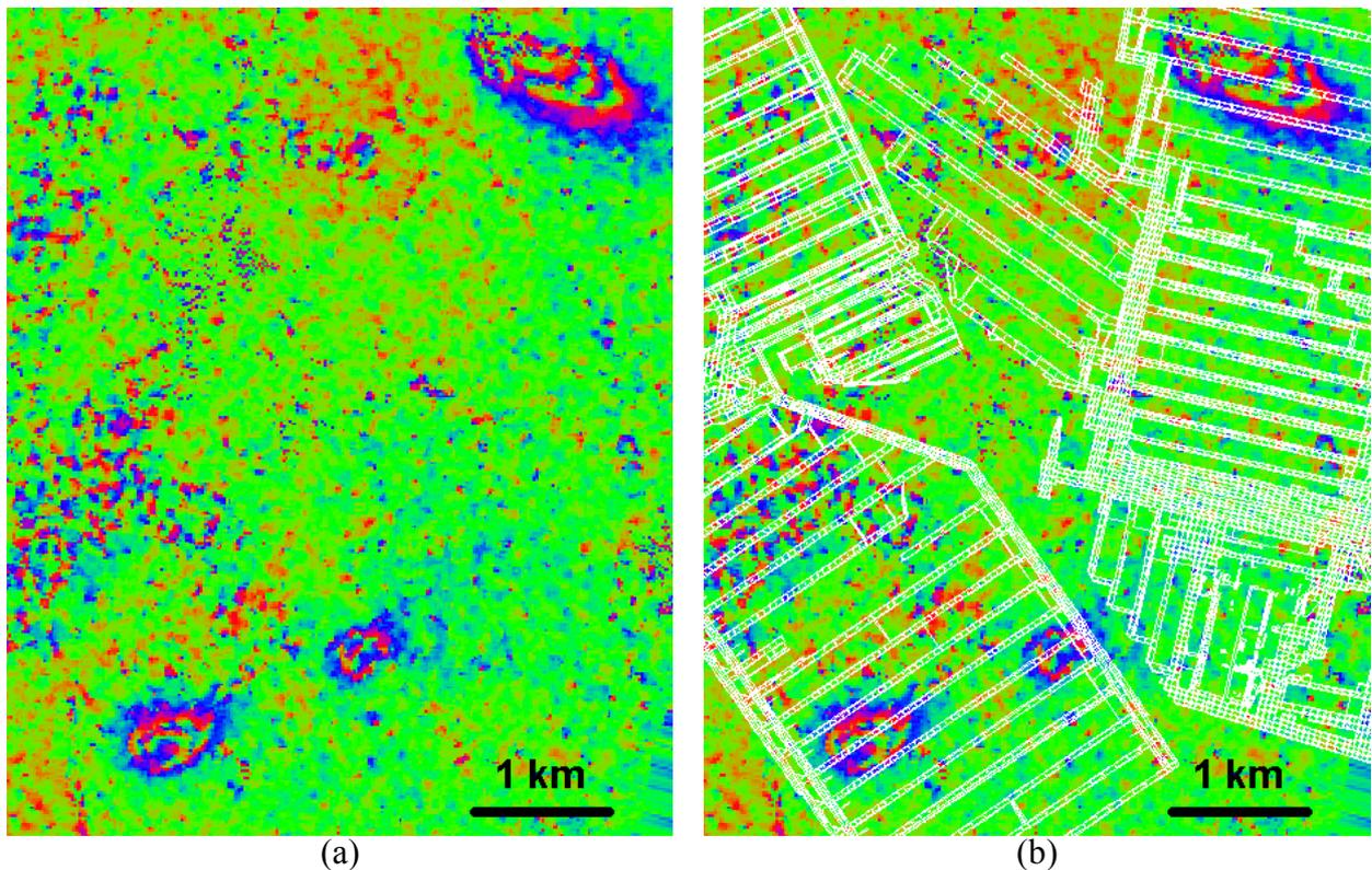
**Figure 5.** (a) JERS-1 DInSAR interferogram showing the subsidence occurred during 09 November 1993 ~ 21 March 1994; (b) same interferogram overlaid with the mine plan.
