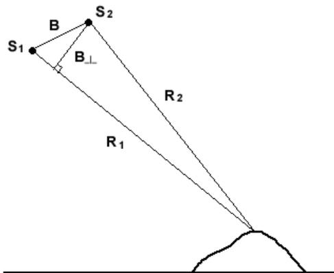
**Figure 1.** Geometry of repeat-pass interferometric configuration.  $S_1$  and  $S_2$  are the locations of the two acquisitions;  $R_1$  and  $R_2$  are the range between the satellite and the ground object;  $B$  is the baseline between  $S_1$  and  $S_2$ ;  $B_{\perp}$  is the perpendicular baseline.
