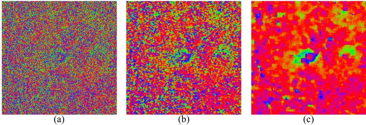
**Figure 4.** The differential interferogram of Radarsat-1 data acquired on 9 October 2004 and 02 November 2004 with a perpendicular baseline of 225m. (a) No filtering; (b) filter window size 2; (c) filter window size 10.
