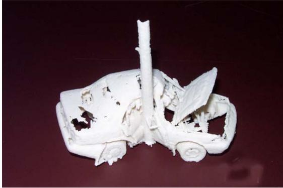
**Figure 8.** Rapid-prototype model of auto accident scene generated by laser scanner data (after Jenkins, 2005)
