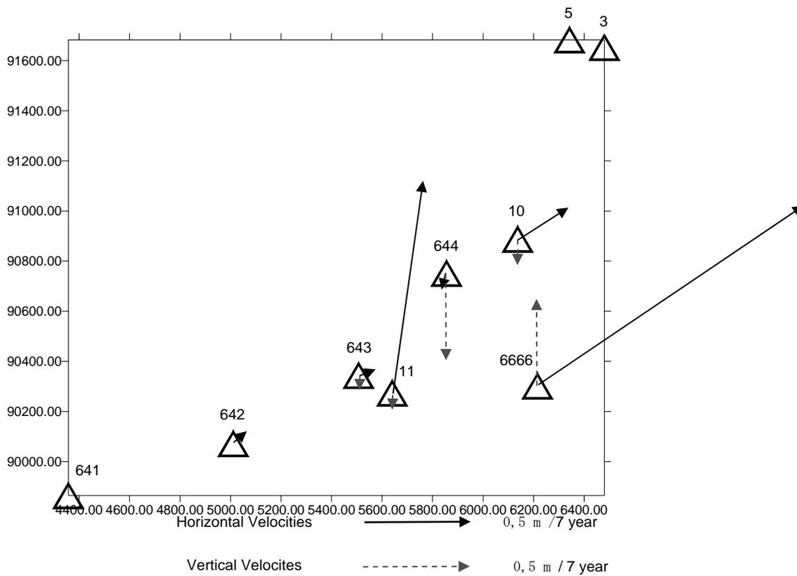
**Fig.9.** Deformation vectors obtained between 1996-2003
