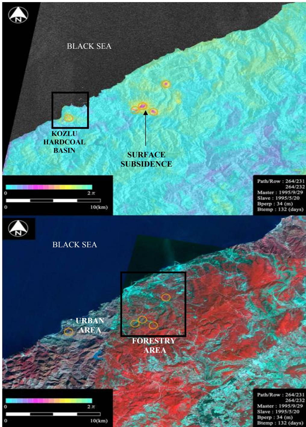
**Fig. 2.** The image above shows deformation surface obtained from JERS-1 satellite. The image below is ASTER infra-red image of the region.
