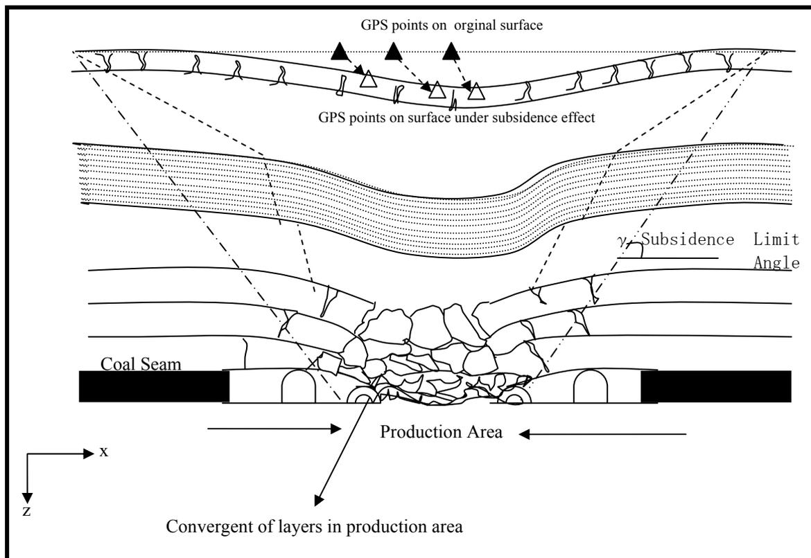
**Fig.3.** Subsidence constitution mechanism in the direction of production (adapted from Shadbold, C. H., 1977)
