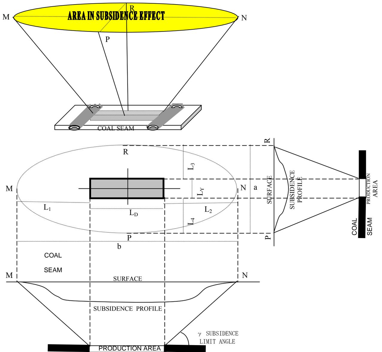
**Fig.5.** Subsidence constitution and its effect area from different profiles in a horizontal seam (adapted from Peng, 1992).
