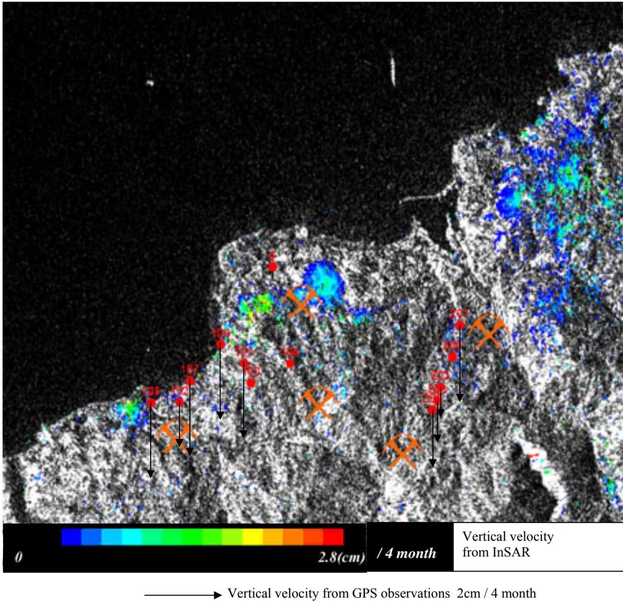
**Fig.12.** Deformation vectors obtained from both methods, GPS and InSAR, in 2005
