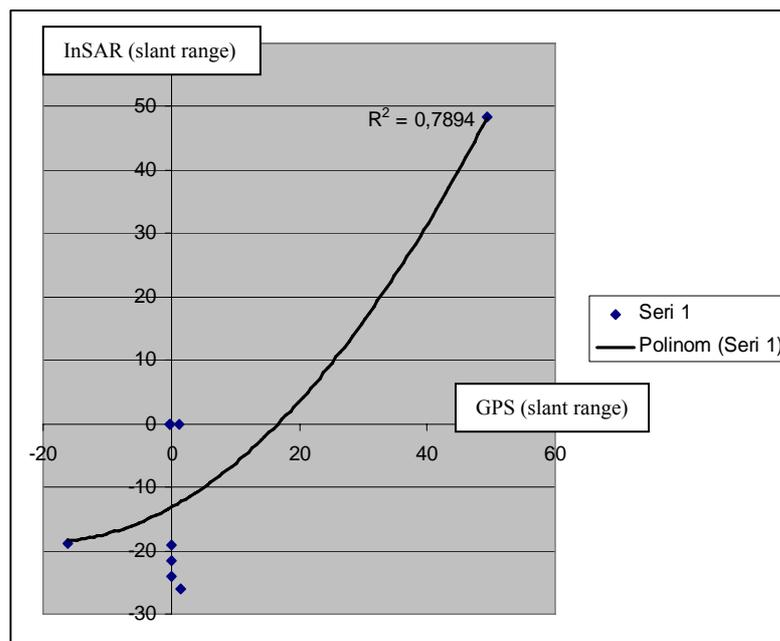
**Fig. 11.** Regression graphics of deformation slant ranges obtained from GPS and InSAR with an interval of 132 days in 1996
