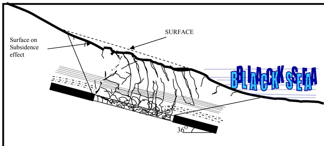
**Fig.4.** Subsidence mechanism in the perpendicular direction of production
