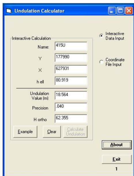
**Fig 7.** The Undulation Calculator Program
