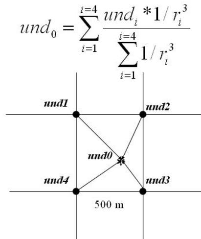
**Fig 6.** Calculation of the arbitrary value with 0.5 x 0.5 km grid
