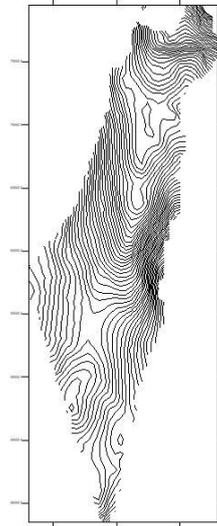
**Fig 4.** The isolines of the geoid-ellipsoid separations
