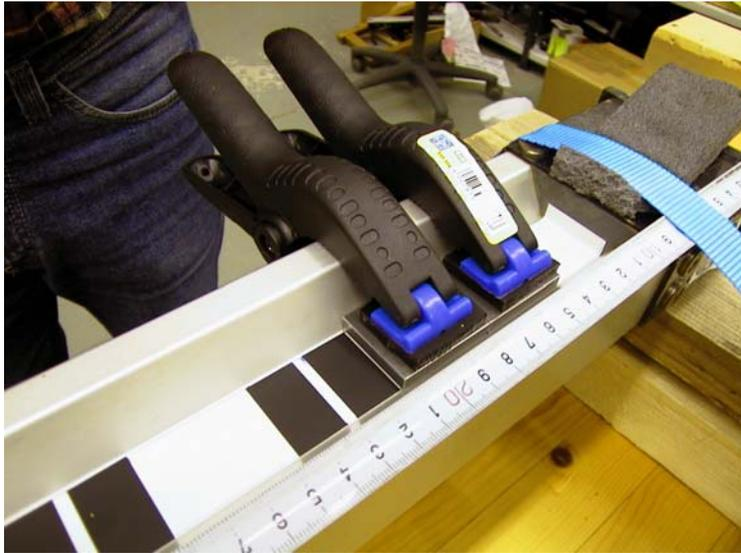
**Figure 1.** Producing of a magnified bar code using precise measuring pieces.
