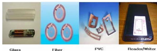
Figure 3.2 Materials of RFID and Reader
