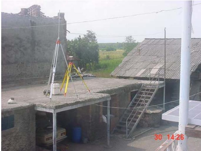
**Picture 2.** DPT-base station on a temporary fix point in the field office of the surveying squad
