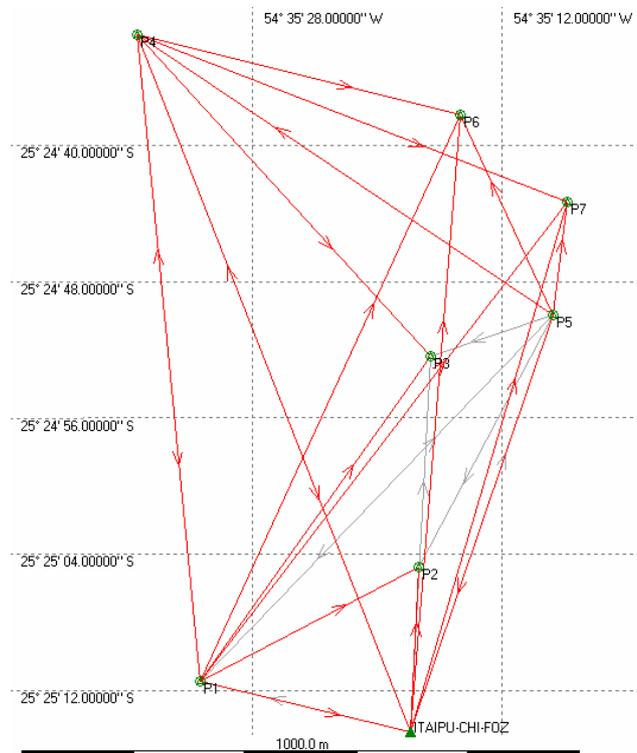
**Fig 4:** Configuration of adjustment network of the pillars P1 to P7 with ITAIPU-CHI-FOZ as a control station
