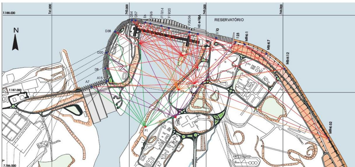
**Figure 1:** Observation pillars and Object Points (ITAIPU DT 2005)
