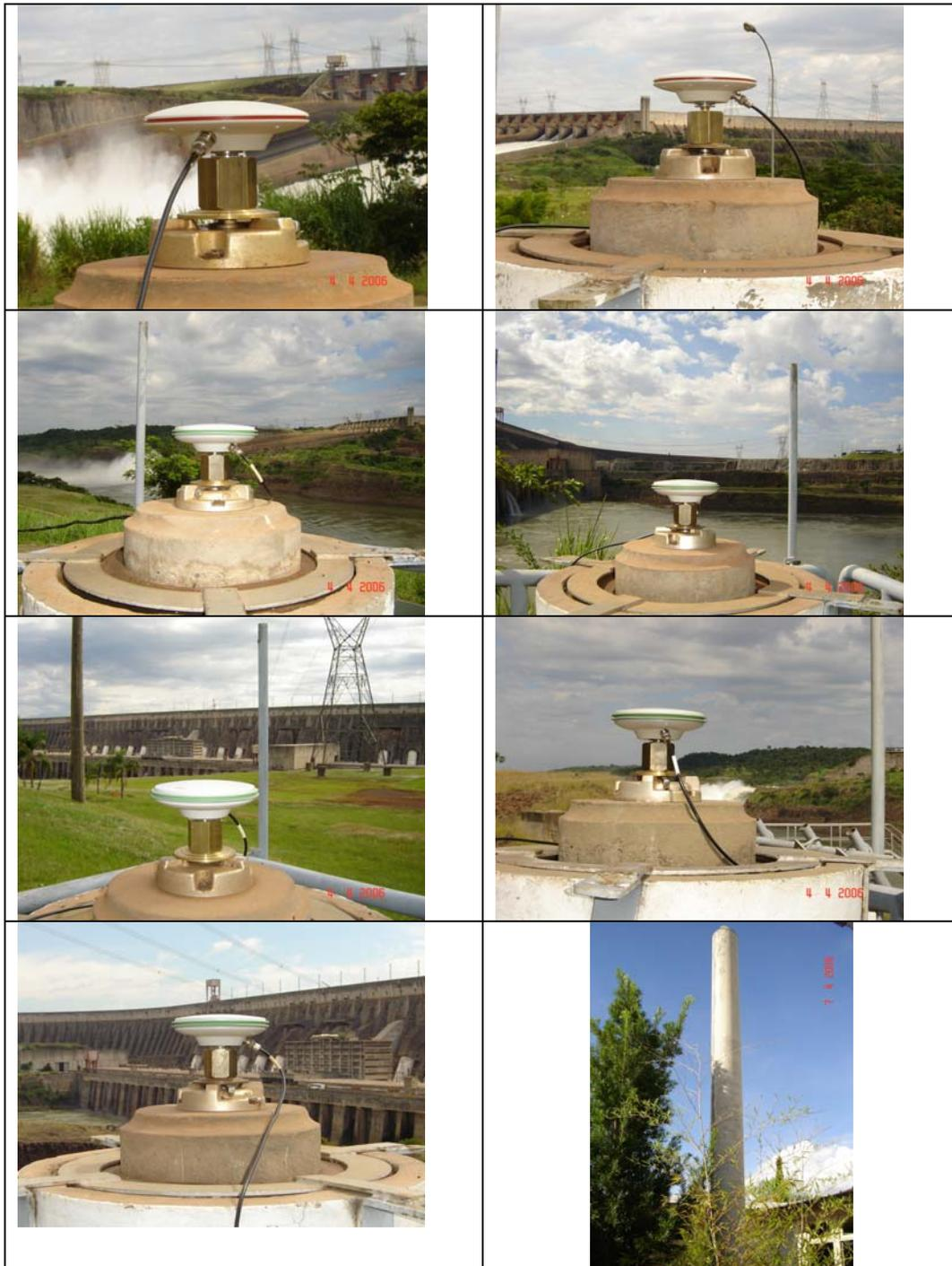
**Fig 2:** Installation of GPS Antennas on top of pillars P1 to P7 and the fix Station ITAIPU-CHI-FOZ respectively
