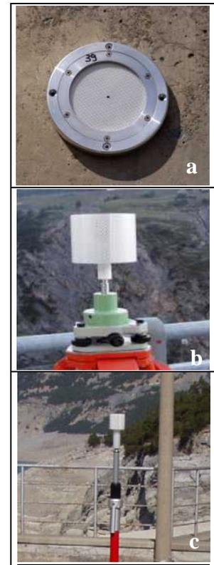
**Figure 3:** different targets used as GCPs
