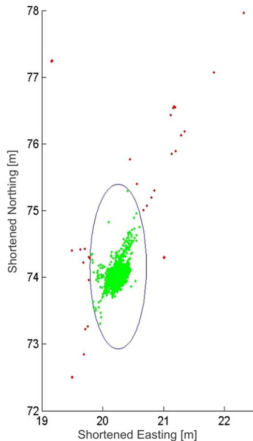
**Fig. 6:** Position of the prism (1 hour) including outliers
