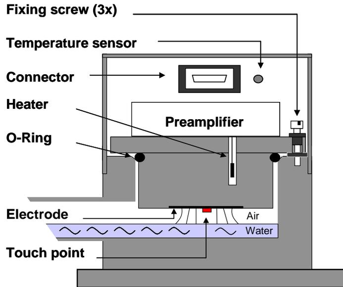
**Fig. 2:** Cross section of a HLS level sensor.
