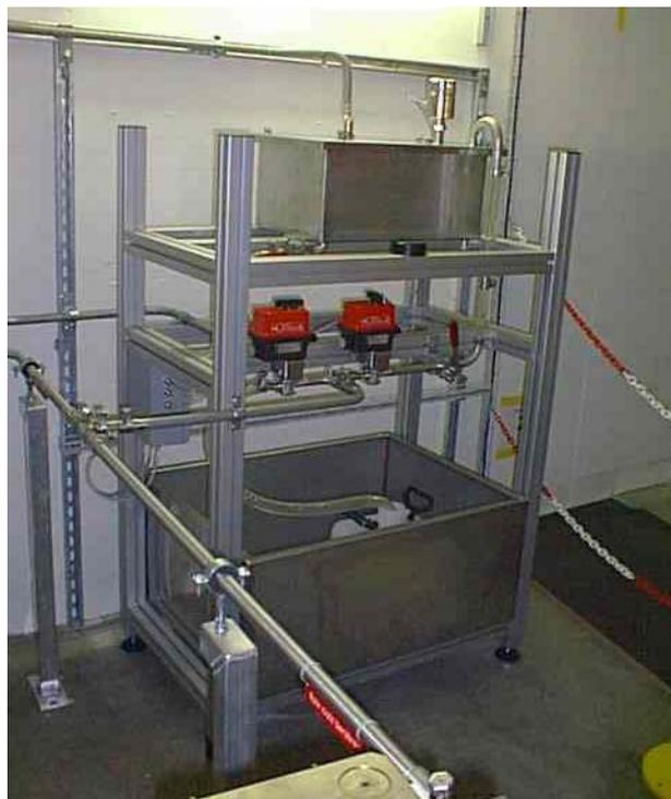
**Fig. 8:** Inner filling station. The two red pumps for draining (left) and refilling (right) of the HLS can be completely remote controlled. The inner filling station is directly connected to the half-filled HLS pipes which can be seen at the lower left corner of this figure.
