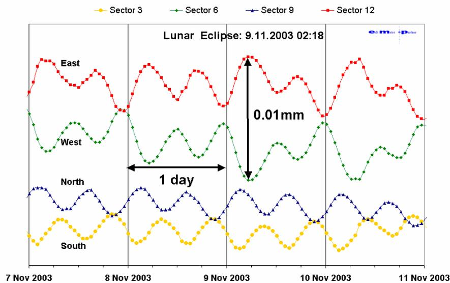
**Figure 10:** A four day period of the year 2003 with a time resolution of 1 hour. The influence of the earth tides with 2 periods a day is clearly visible. Note the high amplitude difference between east and west during the eclipse of the moon.
