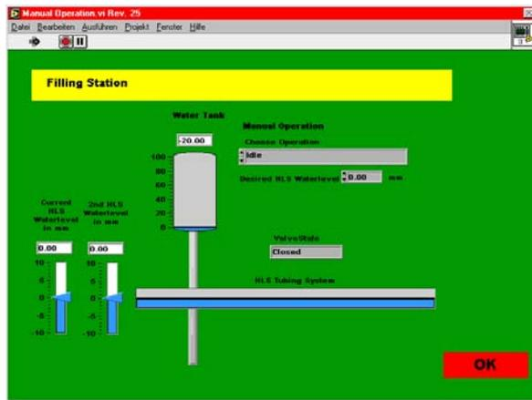
**Fig. 6:** Graphical interface for the automatic refilling station.
