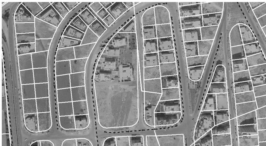
**Figure 13:** Overlay of orthophoto with vector data (DLS-white color; GPS- dotted black)
