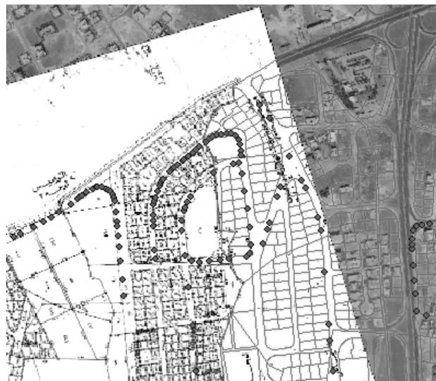
Figure 11: Overlay of best registered map with GPS field survey and Orthophoto
