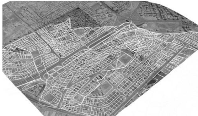
**Figure 8:** 3D view for cadastral boundaries overlaid with Orthophoto.
