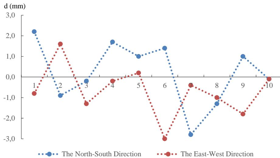
**Figure 7.** The differences between GNSS and the real value
