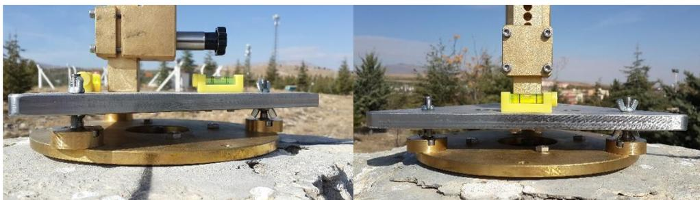
**Figure 5.** Plate levels on the triangular table
