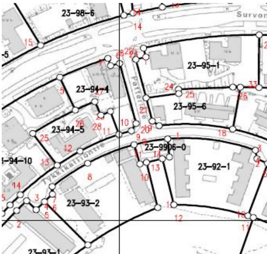
Picture 1. Curved boundary in town plan area. © Maanmittauslaitos, 2017
