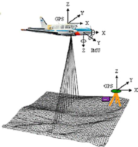
Fig. 1. Laser scanning from an airplane
