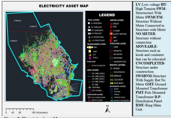
Figure 2: Electricity Asset Map The Impact of Surveying and Mapping in Transforming Ghana's Energy Sector; A Case Study of Electricity Company of Ghana (ECG) Asset Mapping Project (11358) Samuel Larbi Darko and Andrews Kwasi Afforo Odoom (Ghana)
