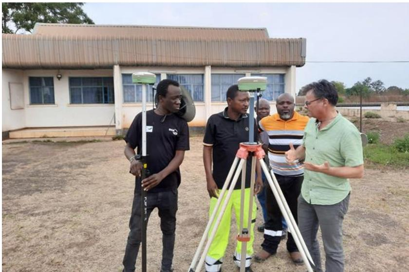
Figure 7: Test measurements with RTK GNSS
