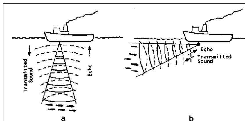
*Figure 4 : Sonar Propagation in water*
