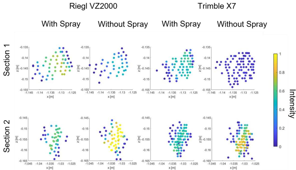
Figure 10: Point clouds with displayed intensities for sections 1 (top) and 2 (bottom) for the measurements with the Riegl VZ2000 and the Trimble X7 with and without scanning array.
