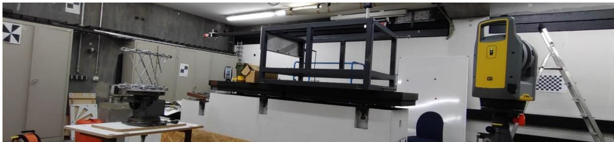
Figure 5: Measurement setup with the object in the initial position and the Trimble X7 laserscanner.
