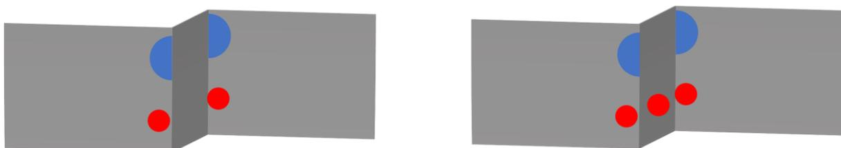
Figure 4: Behaviour of a laser spot on an edge for a time-of-flight scanner (left) and a phase-shift scanner (right).
