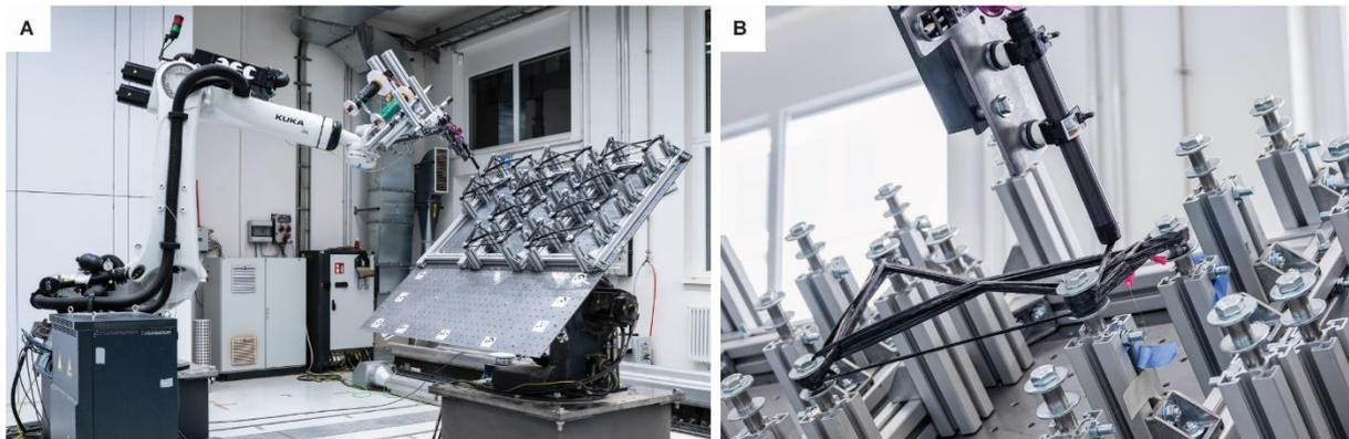
Fig. 2. a) Fabrication set-up with KUKA robot b) exemplary element (Gil Pérez et al. 2022).
