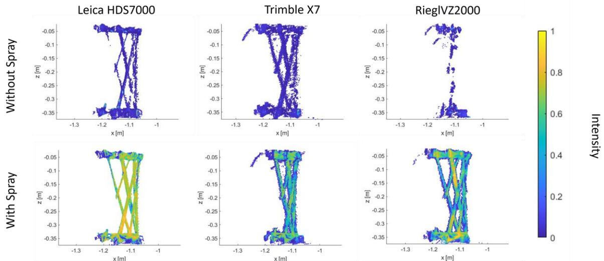
Figure 8: Received point cloud in epoch  $50^\circ$  for all three scanners with and without the use of a scanning spray.
