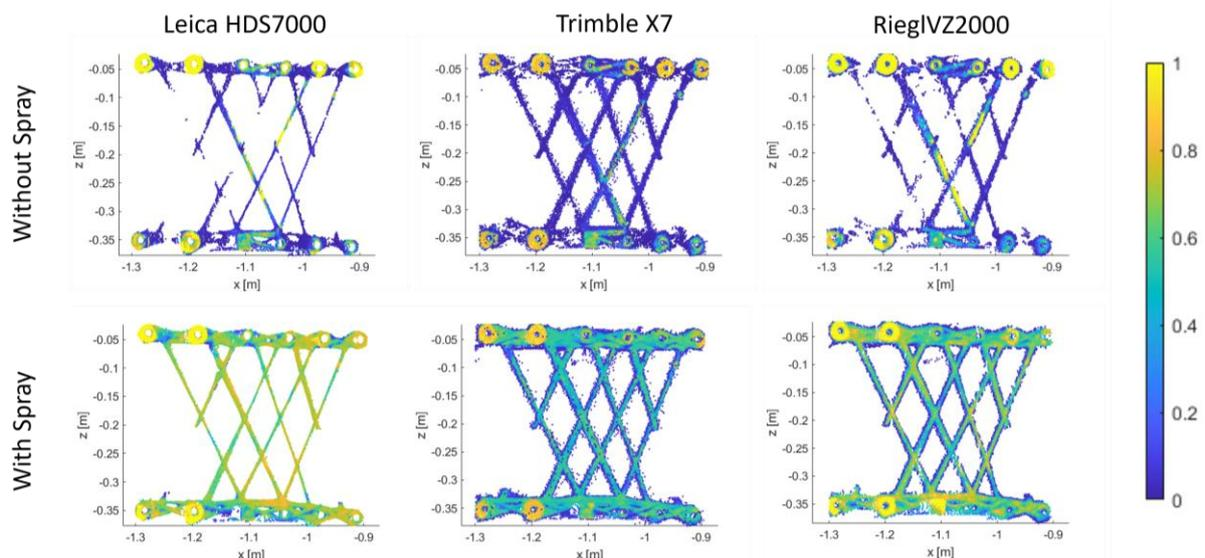
Figure 7: Received point cloud in epoch  $0^\circ$  for all three scanners with and without the use of a scanning spray.
