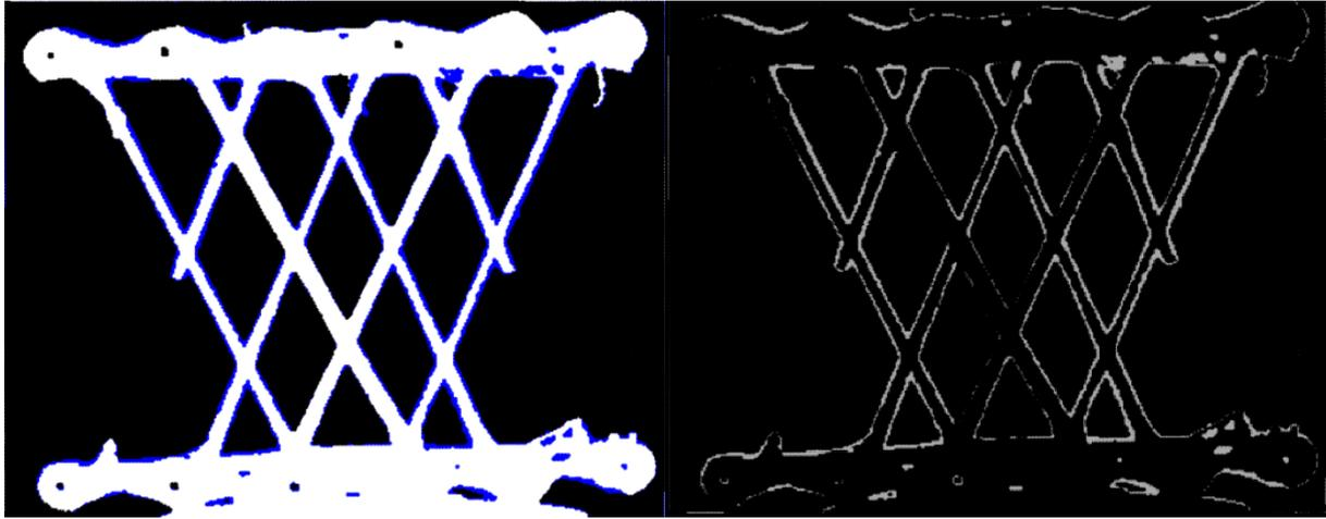
Figure 11: Left: Shadow of both point clouds (Trimble X7 with (black) and without (blue) scanning spray), Right: Difference of the shadow images of both point clouds with the differences in white.
