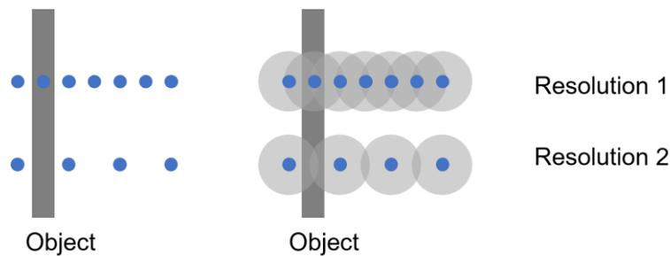
Figure 3: Small measurement object and the measured points in 2 different resolutions. The point centres are shown in blue, while the entire laser spot is shown in grey.
