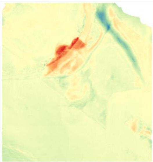
**Figure 5:** The subtraction function was used to identify areas which were more severe. After creating an elevation map in ArcGIS, the red areas showcase the difference in elevation between 1 to 3 metres.
