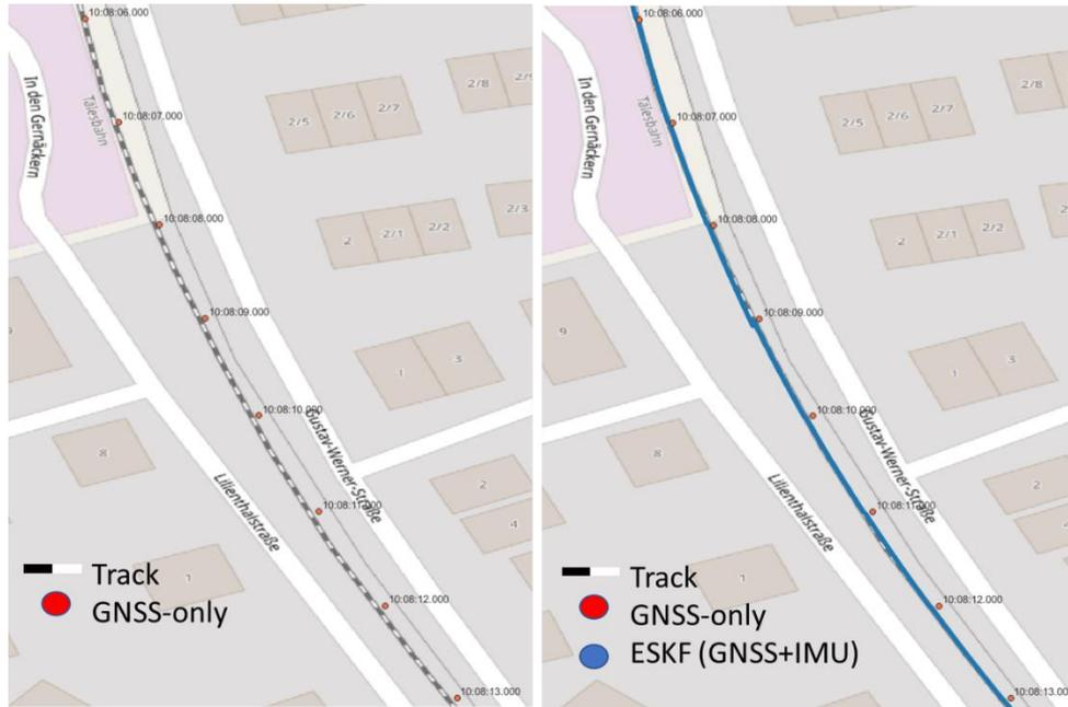
Figure 8: GNSS-only (float solutions) vs. ESKF (GNSS+ IMU) results for one track section
