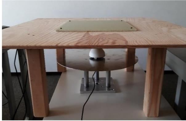
Figure 4: Self-constructed cover plate and GNSS antenna with ground plate (GP)
