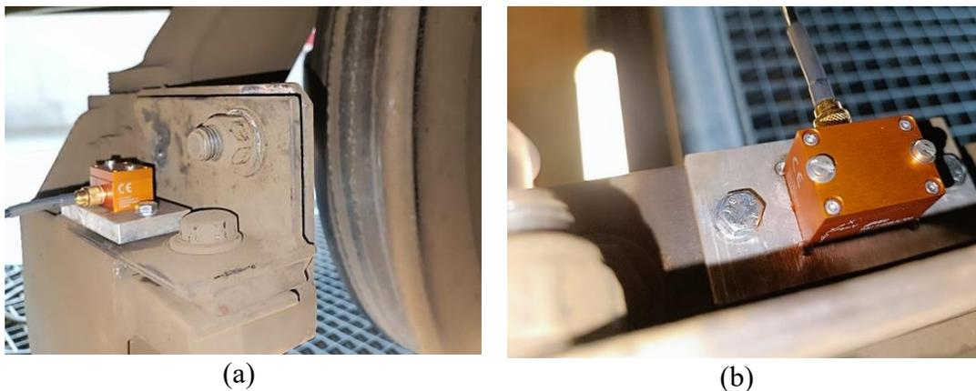
Figure 3: IMU (a) on the bogie and (b) inside the train
