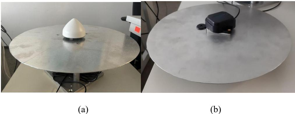
Figure 5: (a) Tallysman TW3972 antenna and (b) u-blox ANN-MS antenna and with GP
