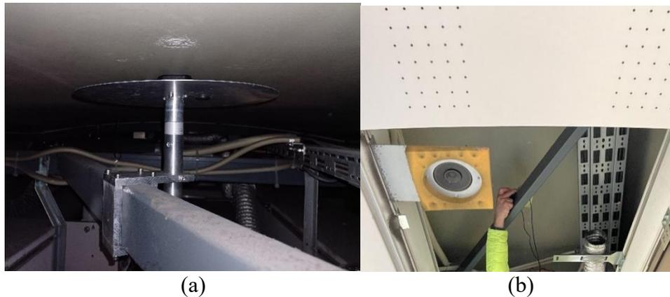
Figure 2: (a) ublox ANN-MS GNSS antenna under the train's roof and (b) antenna vicinity in the train
