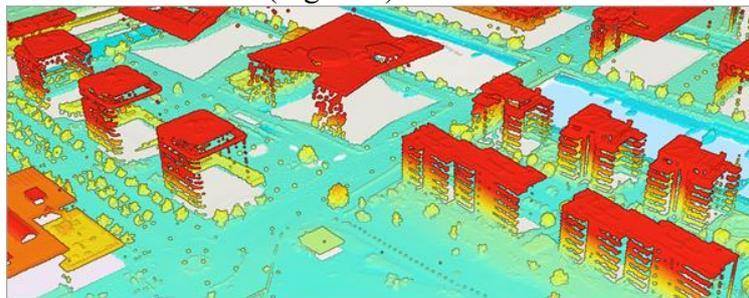
Figure 3: Point cloud LiDAR capture of buildings (Esri 2024).
