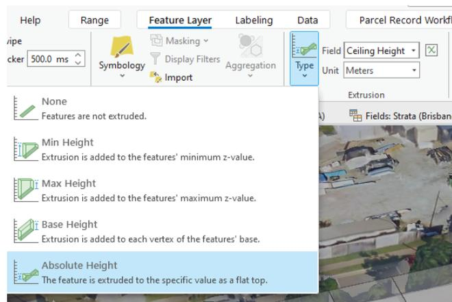
Figure 11: Extrusion of ceiling height to absolute height.
