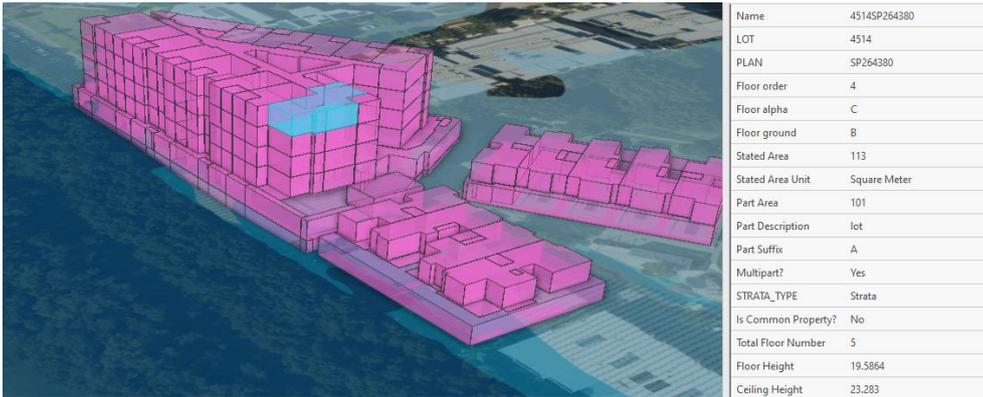
Figure 15: Lot 4514 shown as a 3D Strata unit with height information extracted from LiDAR, overlaid on Brisbane City Council Flood Risk Overall feature service.
