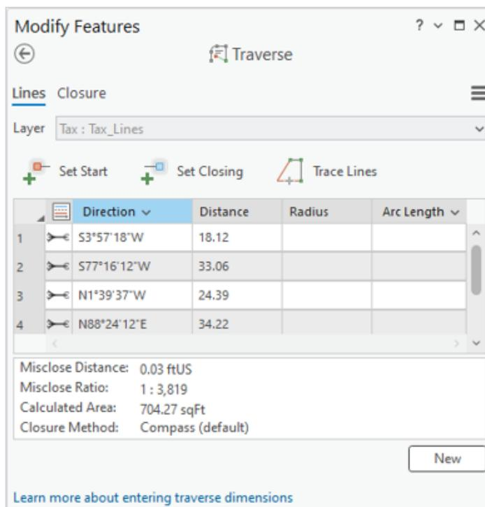
Figure 3: Traverse showing misclose in ArcGIS Pro
