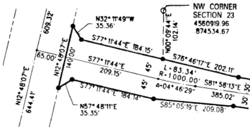
Figure 2: Survey plan showing COGO measurements
