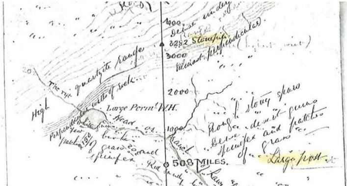
Figure 6 Survey field records of the section north of the 508 Mile post indicating a “stonepile” depicted at the top of a range.
