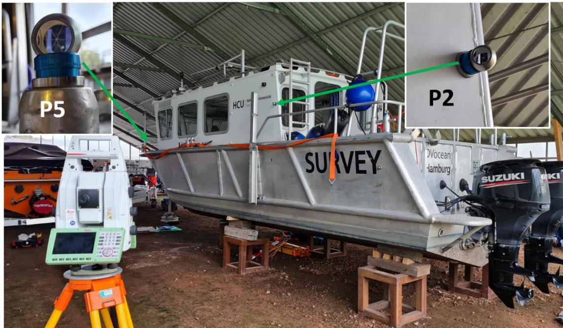
Figure 2: Two fixed points on board the surveying vessel, signaled by SMRs
