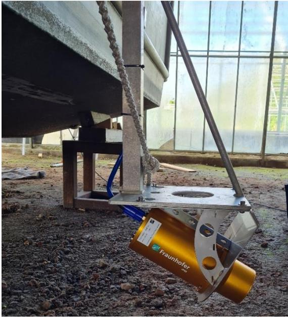
Figure 1: Underwater laser scanner ULi from Fraunhofer IPM
