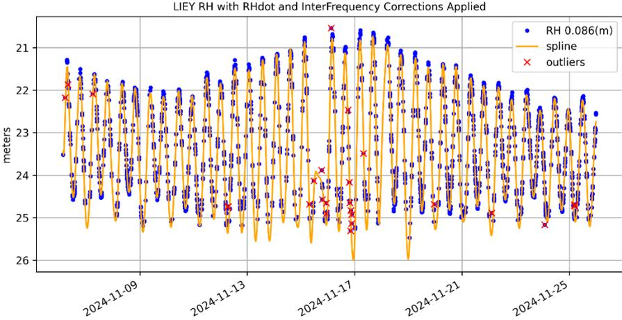
Figure 3: Spline fitting of antenna heights above water after corrections (peak2noise=3.0; Azimuth=135°-270°)
