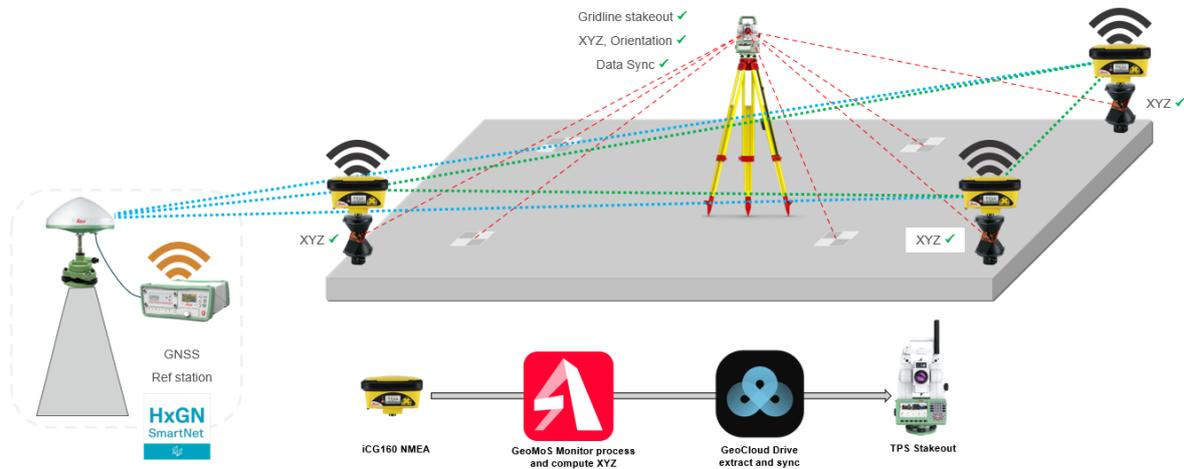
**Figure 4** Core components of the Leica Geosystems' CWCS solution
