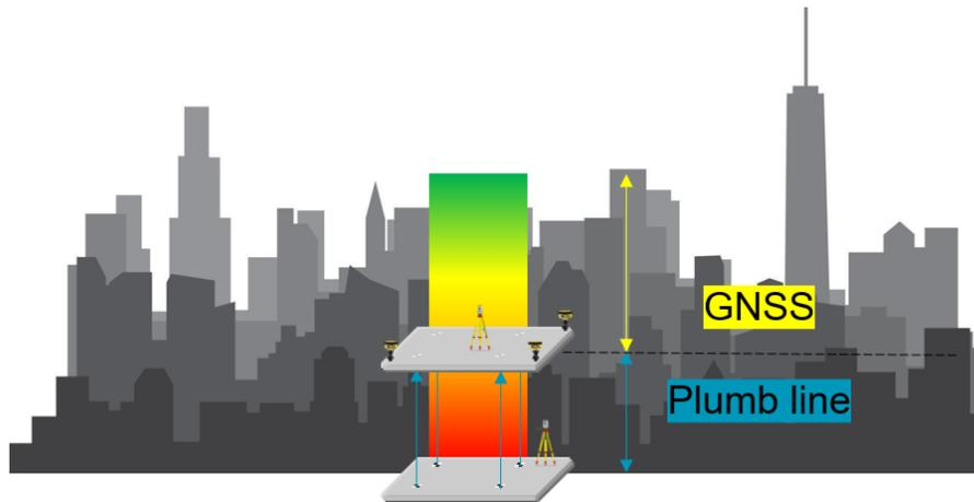
**Figure 7** Positioning solutions for lower and higher levels
