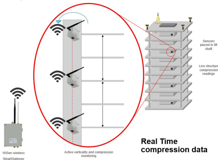
**Figure 5** WiSenMeshWAN® solution for real-time compression readings
