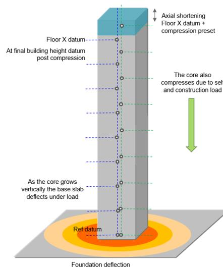
**Figure 2** The effect of the load on tall buildings
